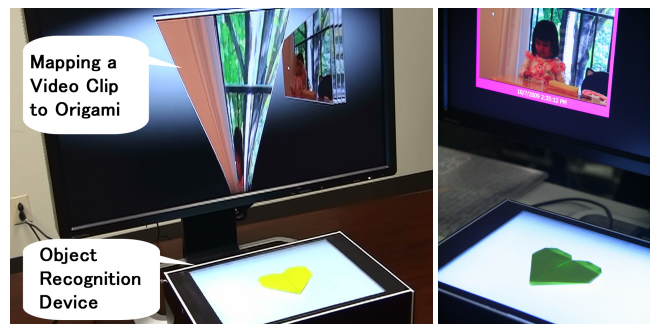
Figure 2: Left: O-Link System's feature to link an object and the related video clips. Right: Play back video clips from an object
